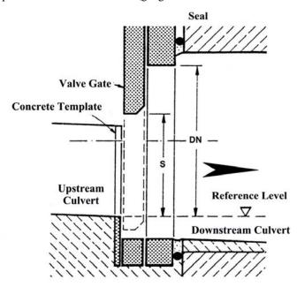
Section through installed HYDROVEX® FluidGate control valve. When closing, the gate takes Figure 3: over the entire closing section, no « pocket » being created.
