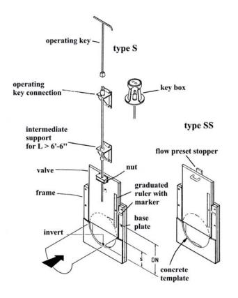
HYDROVEX® FluidGate control valve with extended threaded rod for sufficiently deep chambers type « S », or chambers that are shallow with wedge adjustment, corner type « SS ».
